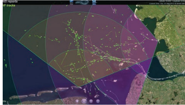
Figure 17: An example of ship tracks resulting from 30 minutes of fused HFSW radar data collected on 1 August 2013.
